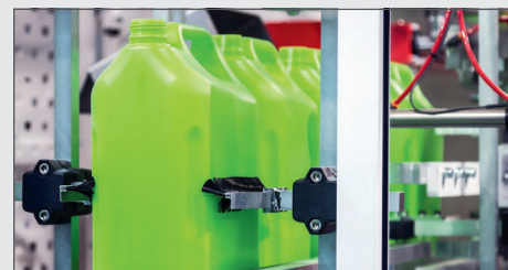
Inline color monitoring of plastic bottles
